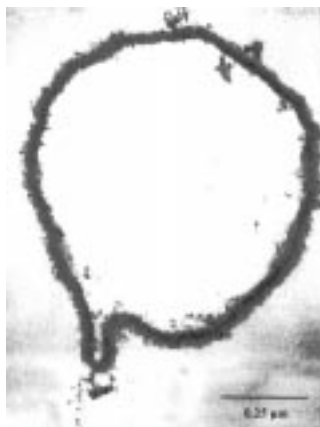
Figure 15. TEM of protein-stained microtome section from sonochemically prepared protein microspheres (Wong & Suslick 1995).
